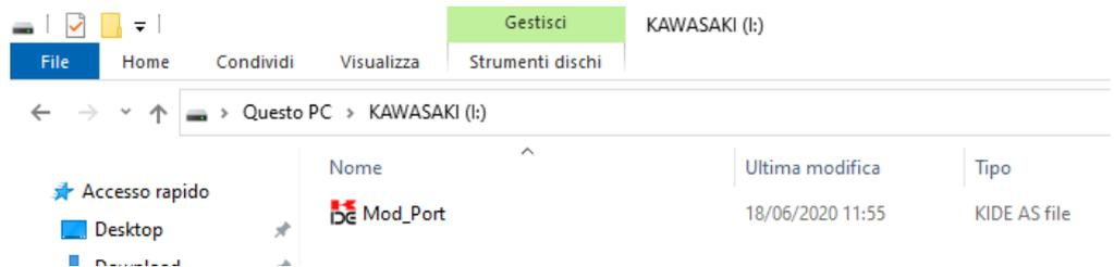
Before being able to use the programs that were transferred, it will be necessary to unlock the communication ports, starting from the 1024. Select the file “Mod\_Port” sent by ARS and copy it on an empty USB memory.
