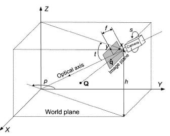
With camera calibration it is possible to get the internal intrinsic (sensor resolution, focal length, lens distortions, ...) and external (position and orientation) camera parameters.
