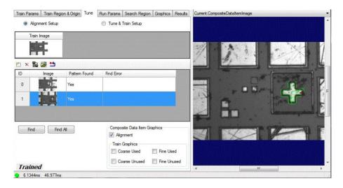
During the alignment setup phase of tuning, you use the controls on the **Tune** tab to manage the collection of **Images** and alignment **Poses** stored within this pattern's **CogPMAlignComposite** object's **CompositeData** collection.
