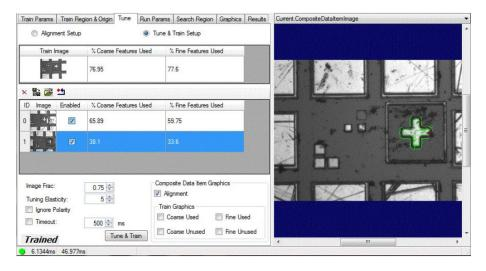
During the tuning phase, you use the controls on the **Tune** tab to configure the tuning parameters, to select which of the images to use for tuning, and to review the tuning results.
