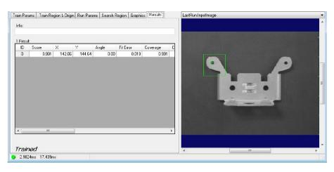
The **Results** tab displays the results of the most recent pattern searches. This corresponds to the **CogPMAlignResult** interface. Use the slider control below the results grid to display the complete set of results.
