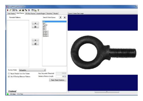
Use the **Multi Params** tab to add and remove the patterns from the Search Order Queue, to reorder the patterns in the Search Order Queue, and to adjust the Multi-Model parameters. For more information on the Multi-Model run-time parameters, see the **Run-Time Parameters Detailed** section.
