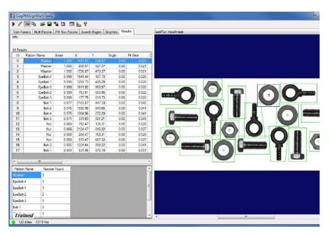
The Results tab is the same as the **Results tab** of the **CogPMAlignEditV2** control but with an extra column to show the name of the pattern and another grid to provide a summary of the results found. This second grid shows the number of instances of the patterns found in the runtime image.
