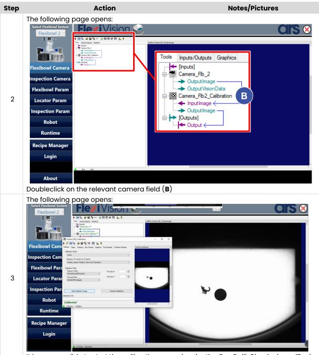
It is now possible to start the calibration procedure by the CogCalibCheckerboardTool.
