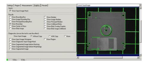
Use the Graphics tab to select what results to see from running the Blob tool. Some of the edit control image buffers appear only if certain types of results are selected. The selections on this tab are equivalent to the modes that can be set with the **LastRunRecordEnable** and **LastRunRecordDiagEnable** properties.
