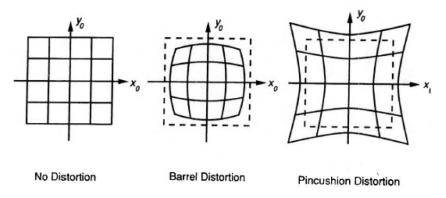
Distortions are produced also by additional filters and the focus/aperture setup.
