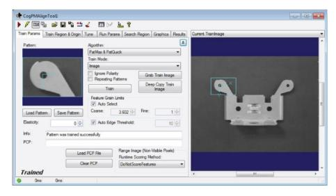
Use the **Train Params** tab to set training parameters and to train the search pattern. Clicking the **Advanced Feature** button so the far right of the tab displays less commonly used features.
