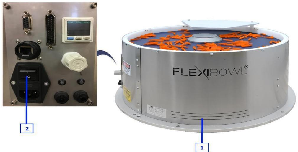
Now simply take an Ethernet cable from the FlexiBowl panel to the robot controller to establish communication.
