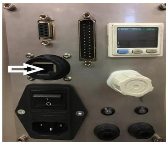
Make sure that the IP address of the robot and that of the FlexiBowl are under the same subnet.
