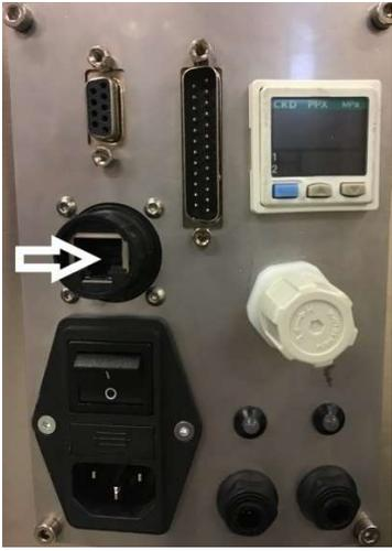
A close-up photograph of a control panel. The panel is metallic and features several components: a D-sub connector at the top left, a vertical multi-pin connector at the top center, a small LCD screen with two buttons at the top right, a white plastic knob in the middle right, and a large black power switch at the bottom center. A white arrow points to a black Ethernet port located on the left side of the panel, below the D-sub connector. |
