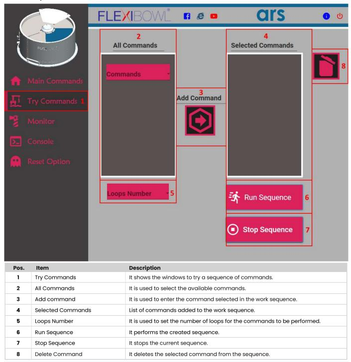
**Note:** To use the parameters set in the previous command windows, you must first save them inside the FlexiBowl®. This can be done in the Option window by pressing the Send Parameters to FlexiBowl® button.
