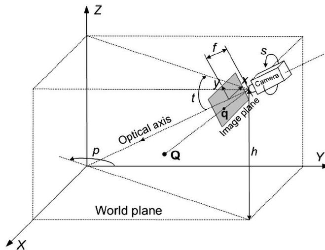
With camera calibration it is possible to get the internal intrinsic (sensor resolution, focal length, lens distortions, ...) and external (position and orientation) camera parameters.
