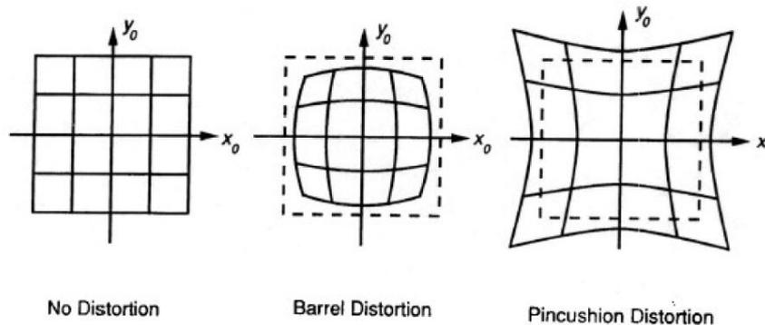
Distortions are produced also by additional filters and the focus/aperture setup.
